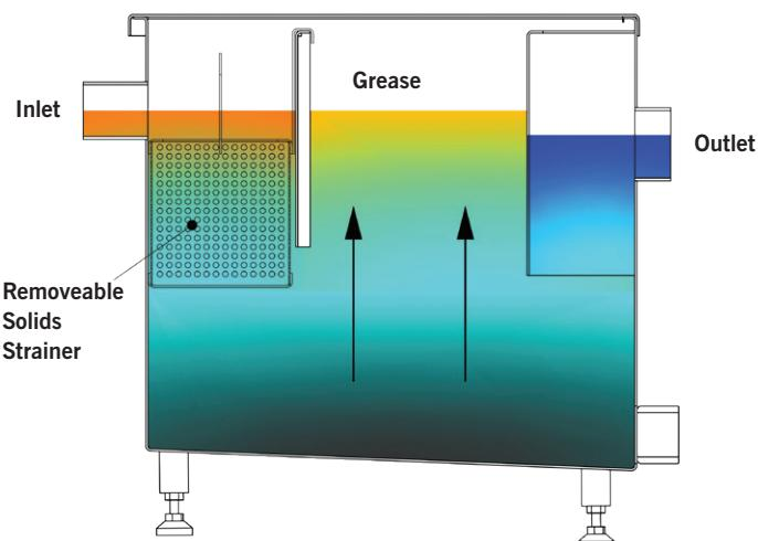
**It is important that the grease separator is sized correctly to allow the waste water to remain for approximately 30 minutes, to ensure the separation process works effectively.**
