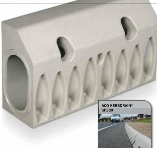
The ACO KerbDrain® 280 splayed range has a profile to match a standard SP kerb stone. The range is ideal for draining medium size catchments such as rural highways and can be easily connected to our 305 half battered range via the use of transition units.
